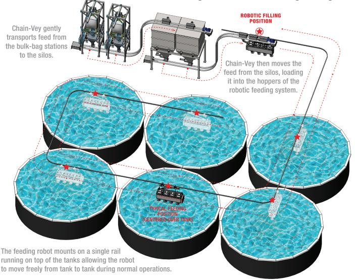
When distributing feed the robot can either stop in the middle of each tank, have multiple feeding points per tank or run along the full length of a raceway giving unparalleled coverage of surface area.
