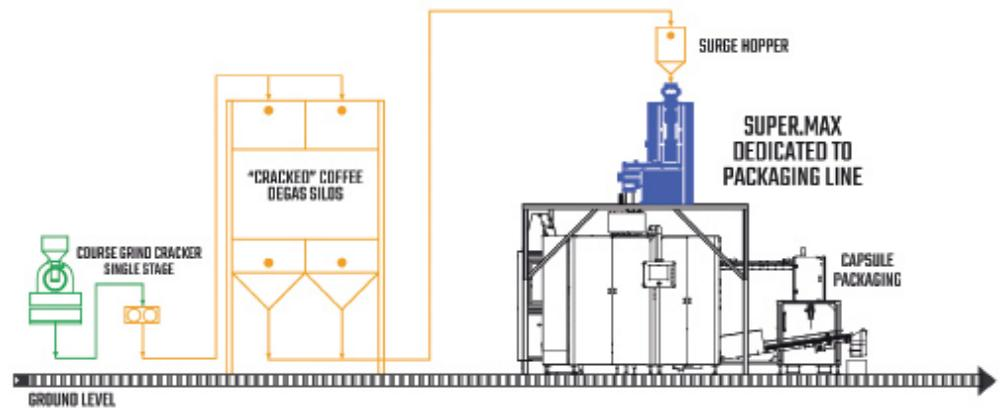
Figure 1: A process flow of a Super.Max installed on top of a capsule filling machine.
