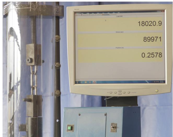
Figure 1: Chain link under a tension load of 18,021 lb before failure.
