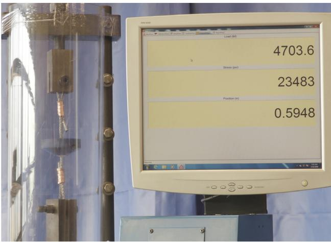
Figure 2: Cable conveyor sample under a tension load of 4,704 lb before failure.
