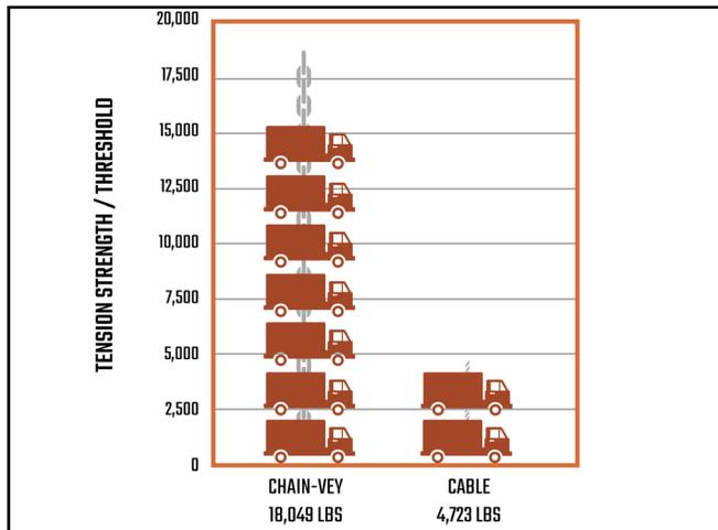
Figure 3: Graph showing the breaking points for Chain-Vey and cable samples.
