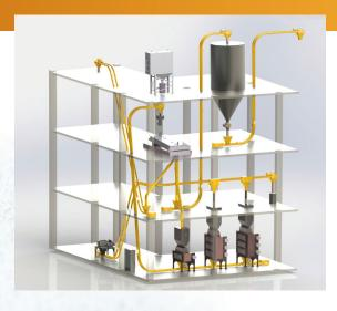
your SAP conveying needs. Its flexible design and compact footprint is sure to fit virtually any configuration. Additionally, with a dust-tight enclosed design, you can be confident your product is protected from the surrounding environment. The MPE Chain-Vey also features Clean-In-Place [CIP] capabilities with automated wash cycles for sanitary conveying needs. Better SAP products require a better conveying solution.
