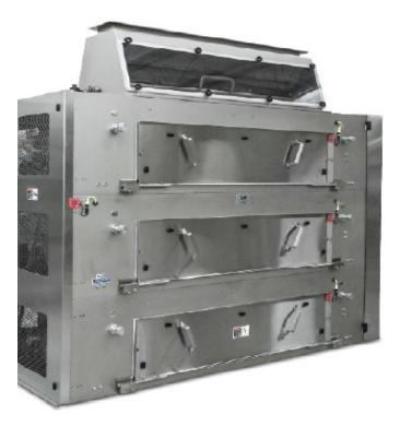
MPE's high capacity Model 1060 Series Roller-Style Gran-U-Lizers provide precisely-controlled uniform particle size distributions, with minimal unwanted "fines", even in the most demanding of applications. The 1060 is designed for industrial food, chemical and mineral processing applications where exact/narrow particle size distributions are desired.
