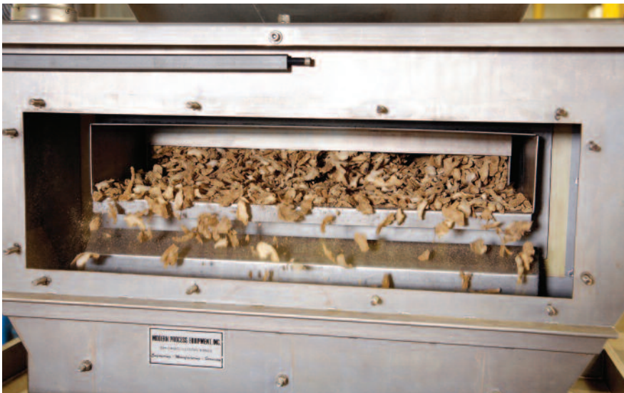
The high-frequency, low-amplitude feeder (shown here with the bolt-on cover’s front panel removed) feeds materials with a wide range of characteristics to the roller mill at uniform feedrates to ensure proper size reduction.
