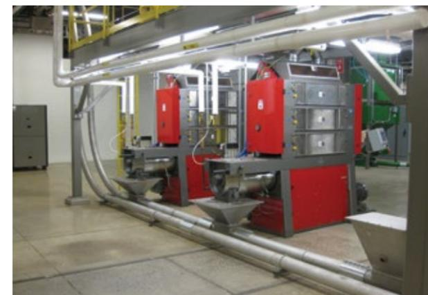
MPE Chain-Vey ground coffee transport system at Melitta Coffee facility. photo courtesy of Modern Process Equipment
