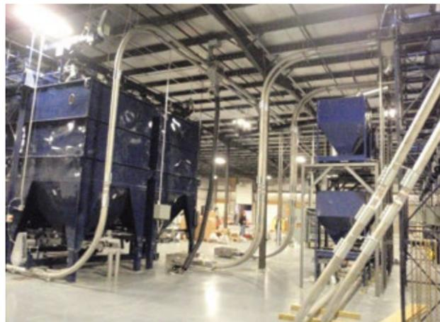
The coffee system at U.S. Roasterie facility uses MPE Chain-Vey conveyors. photo courtesy of Modern Process Equipment
