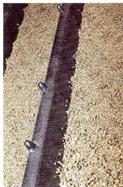
CFB Fluidized Coffee Bed Each individual bean is in suspension and is thoroughly exposed to the heating medium.
